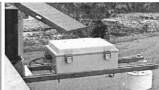
Typical Installation of AWLG over a Bridge
