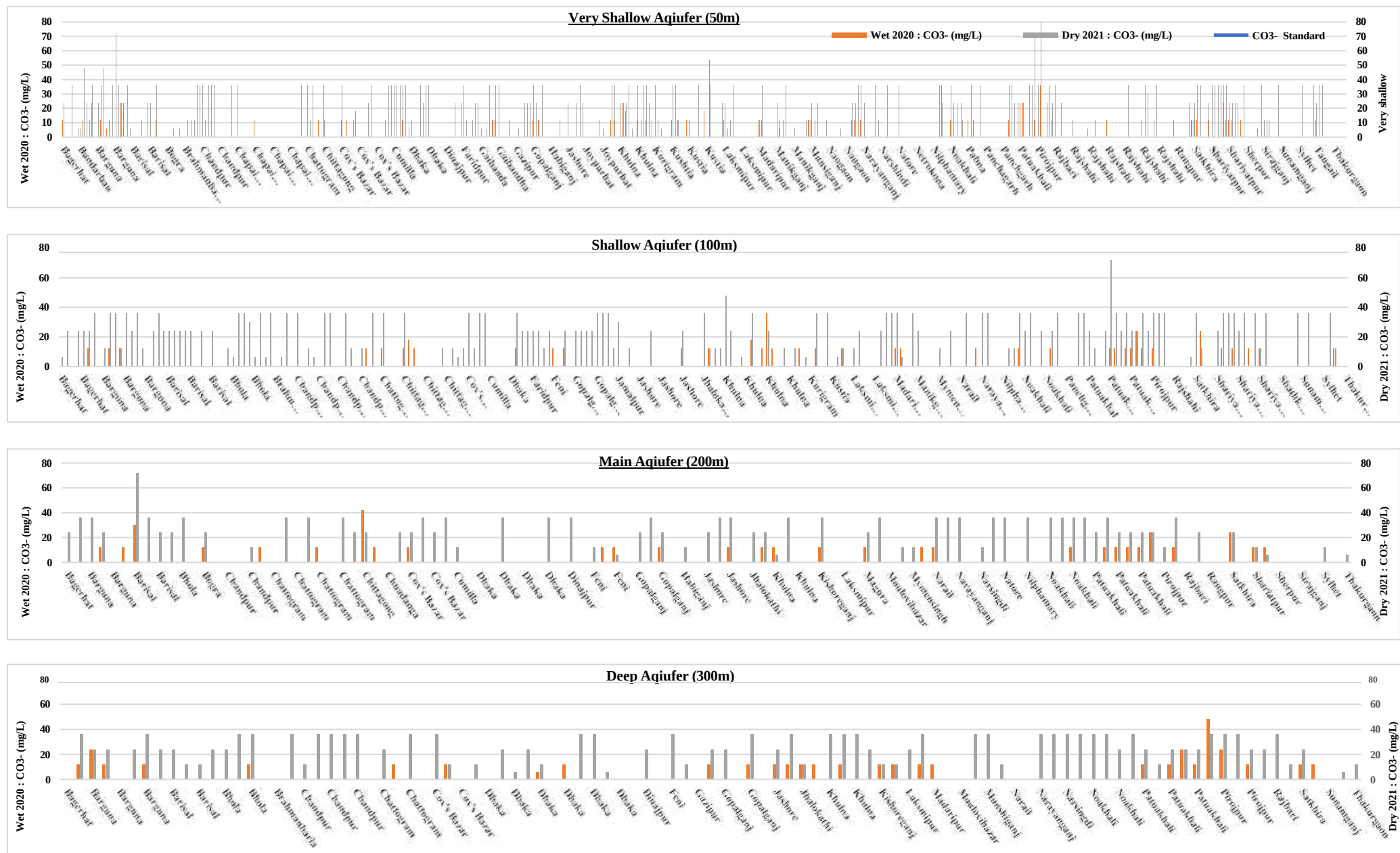
Figure 5-64: Carbonate (CO 3 ) Concentration at Different Depth levels in Bangladesh Groundwater.
