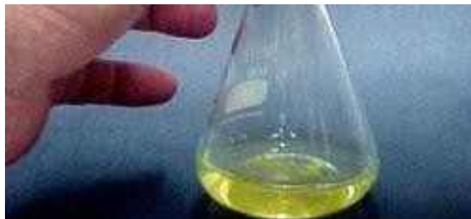
Figure 3-13: After Adding Indicator the Chromate Indicator Colour.
