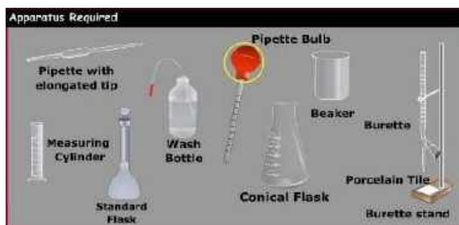
Figure 3-15: Apparatus Required for Carbonate and Bicarbonate Titration.
