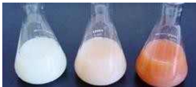
Figure 3-14: Colour Changing Stages with the Addition of Silver Nitrate.
